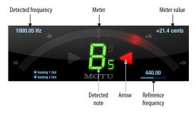
The *Tuner* window is an accurate and easy to use tuner.
