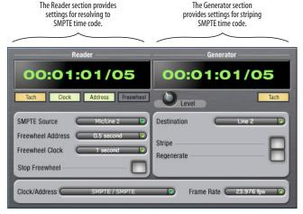
Figure 10-1: SMPTE Setup gives you access to your 4pre's on-board SMPTE time code synchronization features.
