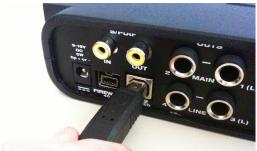
Figure 4-1: Connecting the 4pre to the computer via USB.
