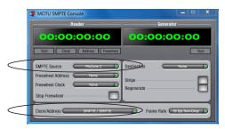
Launch the MOTU SMPTE Console and specify the SMPTE Source, which is the interface receiving the SMPTE time code. Also, confirm that the Clock Source/Address is SMPTE/SMPTE.
