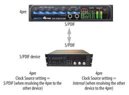
Figure 4-2: The setup for synchronizing a S/PDIF device with the 4pre. Sync is achieved via the digital I/O connection itself. In this case, you have to choose S/PDIF as the 4pre's clock source when resolving it to the other device.
