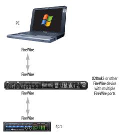
Figure 4-5: Connecting multiple MOTU FireWire audio interfaces.
