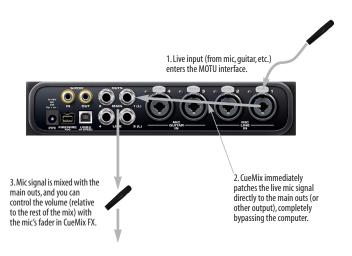
Figure 8-2: This diagram shows the signal flow when using CueMix no-latency monitoring. Notice that this method does not process the live input with plug-ins in your audio software.
