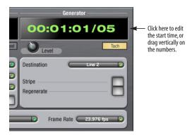
Figure 10-2: Setting the time code start time.
