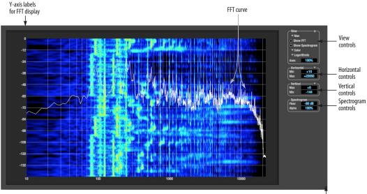
Figure 9-3: FFT and Spectrogram display.
