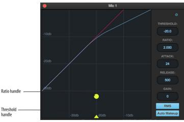
Figure 8-5: The full-size Compressor graph.
