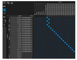
Figure 4-10: Routing Mac channels to physical outputs.
