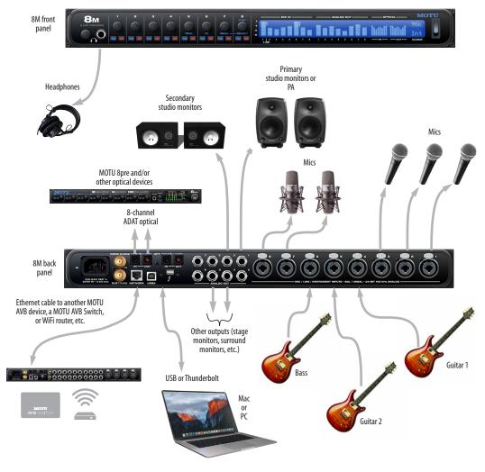
Figure 4-14: A typical 8M studio setup.
