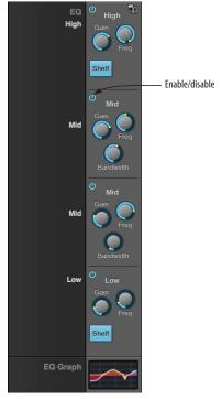
Figure 8-2: The Four-band parametric EQ module.
