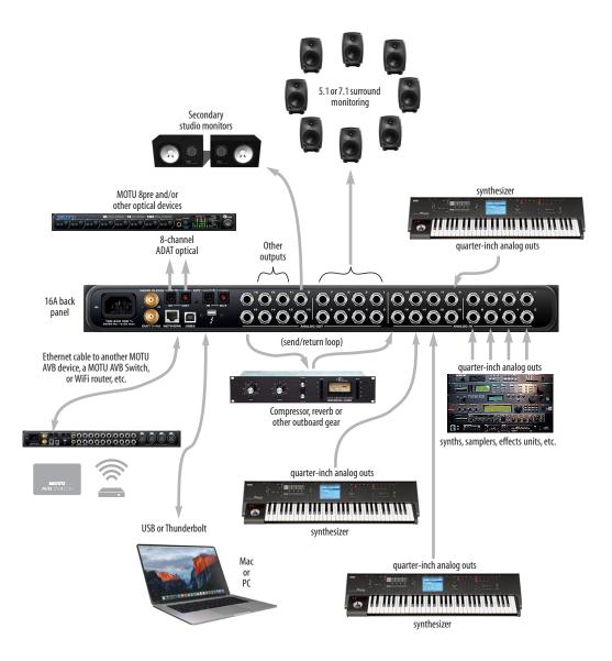
Figure 4-15: A typical 16A studio setup.
