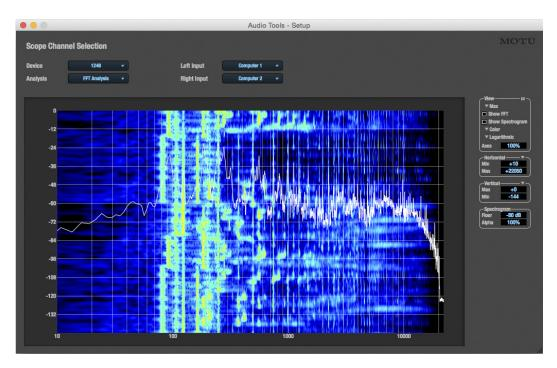
Figure 9-1: The MOTU Audio Tools window with the FFT and Spectrogram Analysis.
