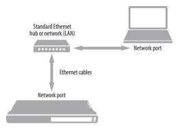
Figure 4-3: Web app control through a standard Ethernet hub or network (LAN).
