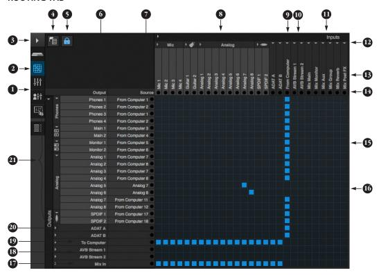
The Routing Tab lets you route inputs to outputs. Outputs are listed by row on the left; inputs are listed in columns across the top. Simply click in the grid to make a single connection. Click and drag to make multiple connections in one gesture. To route a single input to multiple outputs, make multiple connections vertically in the same column below the input. To mix multiple inputs to the same output, you'll need to use the mixer (page 22) and the Mix In bank in the routing tab (17).
