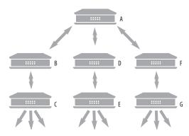
■ AVB audio can't pass through more than seven switches. However, you can daisy-chain more than seven switches and route audio freely among them. You just won't be able to create point-to-point connects that span more than seven switches.
