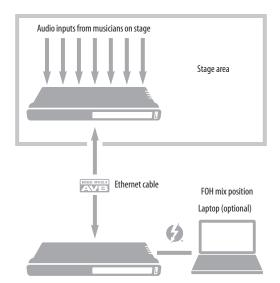
Figure 5-4: Use the Stage I/O preset to connect audio inputs and outputs to other AVB devices on the rest of the network.
