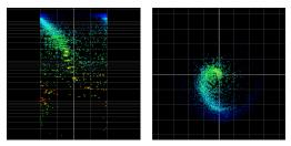
Figure 9-27: A stereo mix with phase issues.
