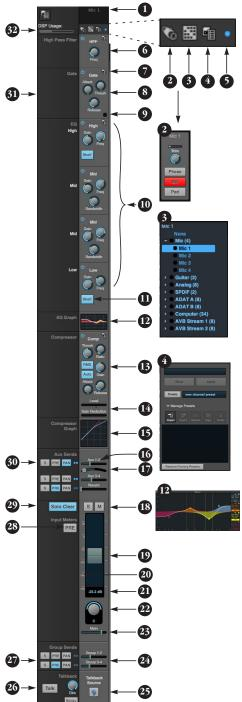
To access a mixer input channel strip, go to the Mixing tab (page 22), reveal the side bar (item #3 on page 22), and show the input channel in the Mixer Inputs section (31). To show and hide sections of the channel strip, such as EQ or the compressor, use the Controls section of the side bar (item #3 in the Mixing tab on page 22).
