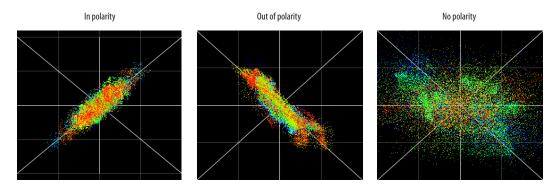
Figure 9-18: Checking polarity in a stereo signal with the X-Y Plot.
