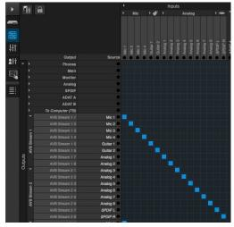
Figure 4-11: Routing physical inputs to the Mac.
