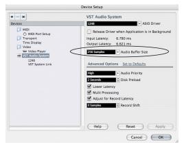
Figure 7-3: In Cubase or Nuendo, choose Devices menu > Device Setup. Select your interface (1248, 8M or 16A), then click the Control Panel button to access the window above and the Buffer Size setting.
