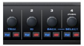
Figure 6-2: Push the knob to activate the functions labeled in blue.
