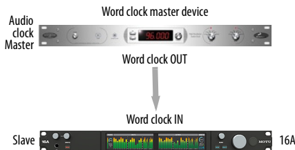
Figure 4-5: Slaving the 16A to word clock. For the 16A clock source, choose Word Clock In .
