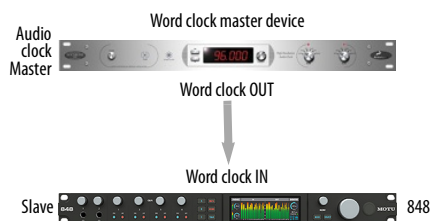
Figure 4-7: Slaving the 848 to word clock. For the 848 clock source, choose 'Word Clock In.'
