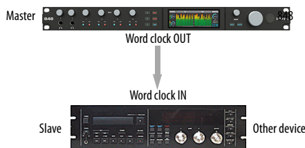
Figure 4-6: Slaving another digital audio device to the 848 via word clock. For the 848 clock source, choose Internal (or any source other than Word Clock , as daisy-chaining word clock is not recommended).
