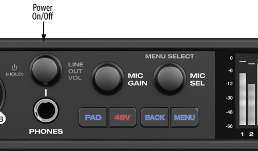
Figure 5-2: Push the knob to activate the functions labeled in gray.
